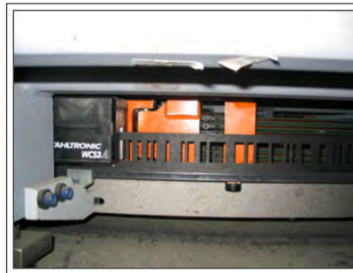
In-Floor pit which houses the electrified rail system as well as the position strip. A rabbit device reads the location strip and picks up power from the rail and delivers it to the system
