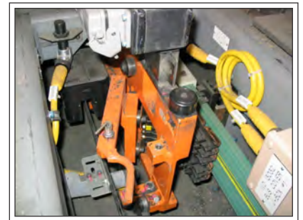
In-Floor pit which houses the electrified rail system as well as the position strip. A rabbit device reads the location strip and picks up power from the rail and delivers it to the system
