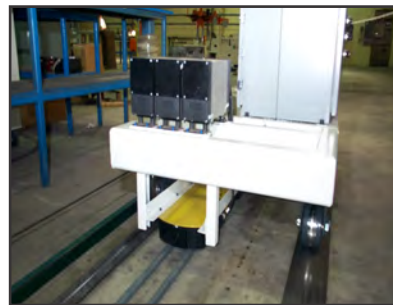
Non-contact inductive power with pickup device on the cart
