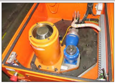
Product: Servo Lift / Level Arbor Capacity: 8,000 lbs / 3,629 kg Lift Stroke: 8 in / 203 mm
