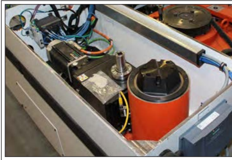
Product: Locking Lift Arbor Capacity: 14,500 lbs / 6,577 kg Lift Stroke: 8 in / 203 mm
