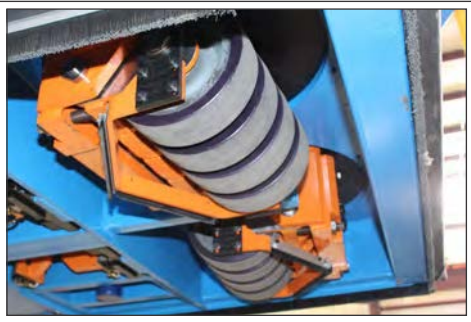
Product: Quad Wheel Suspended Caster Capacity: 19,000 lbs / 8,618 kg
