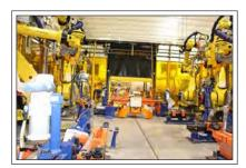
Fori recently supplied a high volume, flexible automated adhesive apply, robotic drawn arc stud welding and robotic spot welding system consisting of two identical lines and a state of the art, RGC (rail guided cart) system for part transfer.
