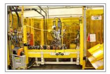
Fori recently design and built a low volume nut welding & spot welding cell for hot stamped materials. Maximum utilization of floor space and capital equipment was accomplished by batch running right or left hand door rings.
