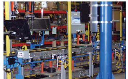
**Fori Automation's latest assembly line consists of several modular sections, each of which features a master I/O distributor that is fieldbus independent and vendor neutral. Photo courtesy Balluff Inc.**
