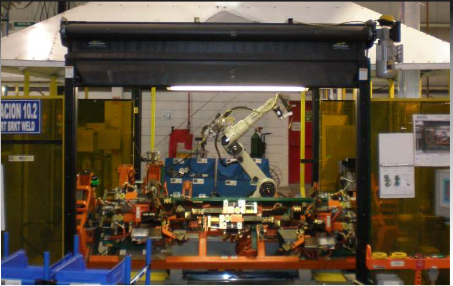
Automatic welding cells with main axle automatic press and geometric locating fixture with one MIG welding robot, MH transfer robot with holding position for MIG robot pickup.
