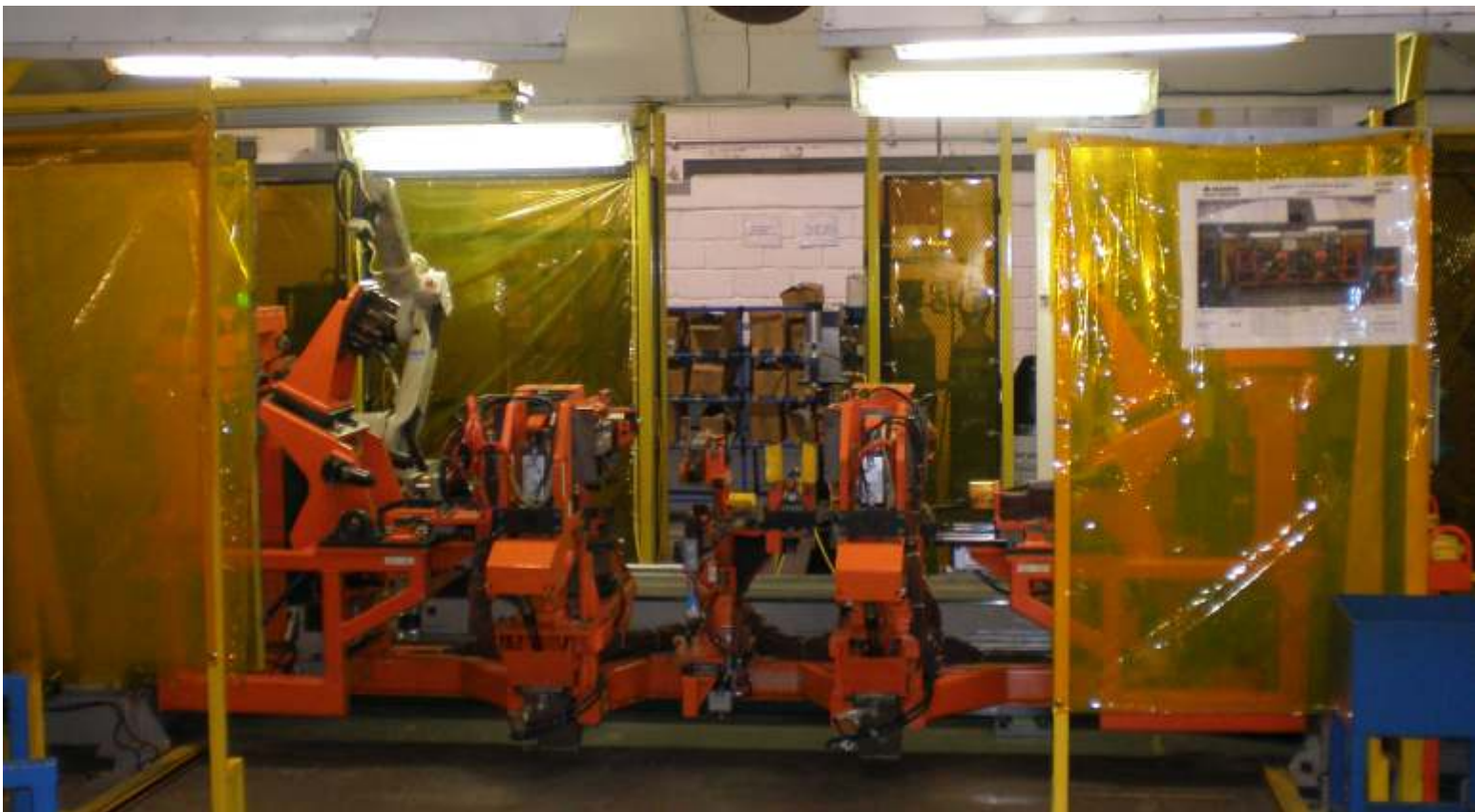
Automatic welding cells with main axle automatic press and geometric locating fixture with one MIG welding robot, MH transfer robot with holding position for MIG robot pickup.
